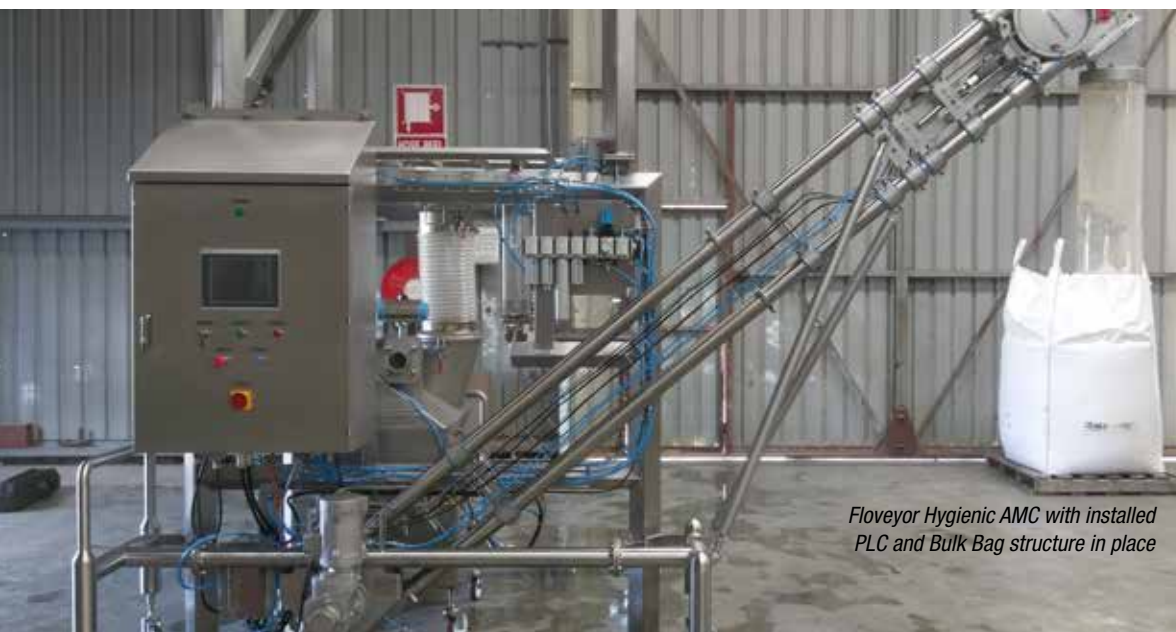
Floveyor AMC for beverage manufacturing customer with custom hopper and dust containment system showing full system with NORD motor installed.
